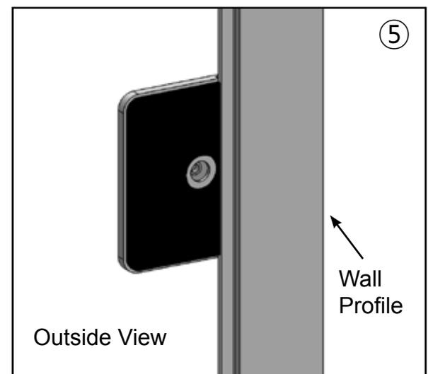
1. Dismantle the Wall Brackets and fit onto the Panel Glass ensuring that all gaskets are fitted. Ensure that the brackets are fitted the correct way (screws to the inside).
