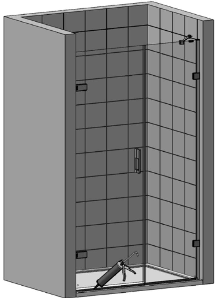
1. Place the Bracing assembly onto the top of the Panel Glass and up to the tiled wall, use a Spirit Level to keep it horizontal.
