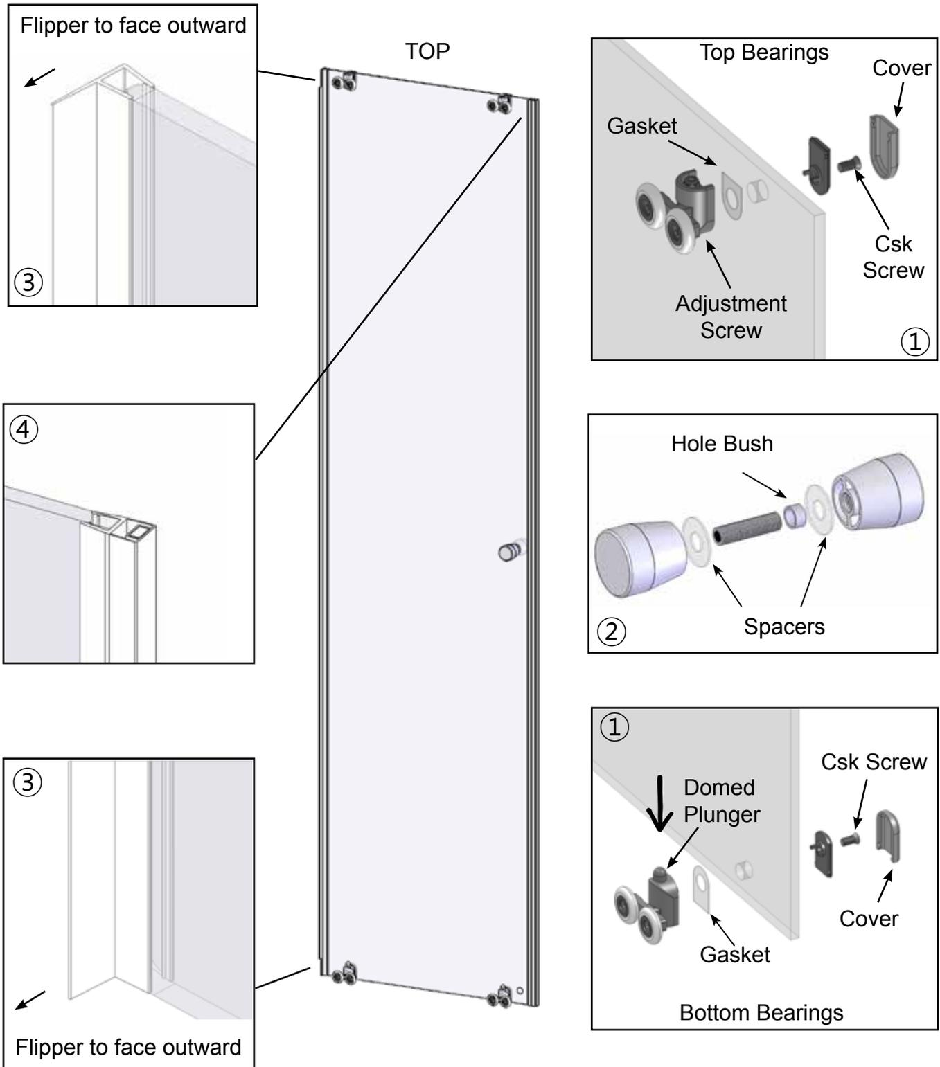
1. Carefully dismantle the Bearing Assemblies, place the gasket on the outside of the glass (Bearing Side) then re-assemble onto the Door Glass. Make sure you have the correct bearings at the top and bottom and that the wheels are on the outside of the glass.
