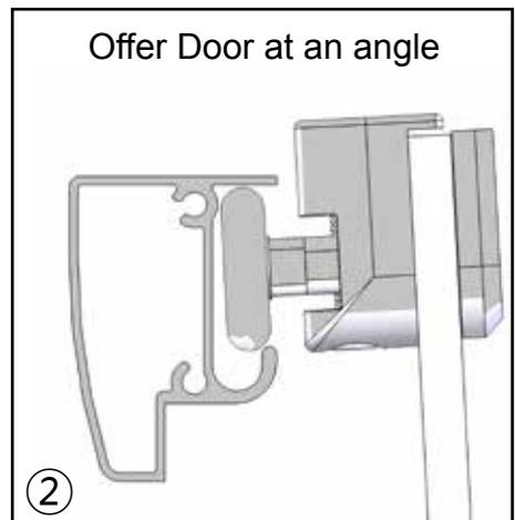
1. Carefully lift the assembled door into the enclosure ensuring that it is the correct way round.
